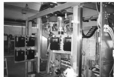
Illustration 1.13: Decentral motor controls integrated in packaging machine
