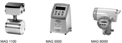
Sensor housing and flanges are designed in carbon steel (ASTM A 105) and terminal box in fibre glass reinforced polyamide or optionally in stainless steel (AISI 316). Measuring pipe is made of stainless steel (AISI 304) while liners and electrodes are available in various materials, making the sensor highly resistant to a wide range of chemicals.
