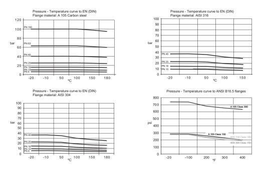
Table 8-14 Metric measures (pressure in bar) - Sizes 25 mm, 40 mm and >300 mm
