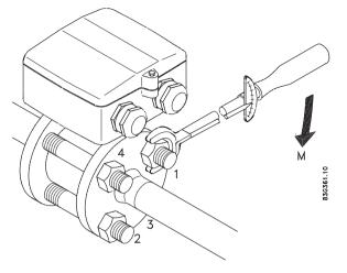
The bolts must be tightened using up to 50% of the max. tightening torque for the pipe dimensions stated. The max. tightening torque for different size pipes is given in the table.
