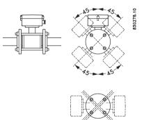
Figure 4-6 Horizontal installation, various terminal box positions
