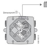
4. Fit the  $\frac{1}{2}$ " NPT or M20 cable glands for supply and output cables.
